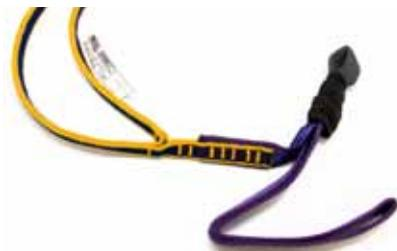
3 - At the lanyard end, check on each side of the webbing that there are **5** yellow bar tacks connecting the tear webbing to the blue & yellow lanyard components\*.
